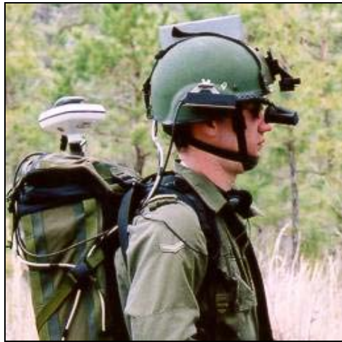
Figure 1: TekGear M1 Personal Viewer HMD used for static visual mode studies.
